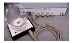
Connect the transducer interface (EIPF) to the main unit using the 8 pin mini DIN cable
