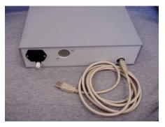
Connect the main unit to a USB port of the host using USB cable.
