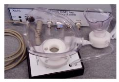
Connect the nasal mask to the transducer interface channel 3 (nasal flow) using nylon tubing. The transducer connection is inside the unit to protect it. Care must be taken when connecting the tube.
